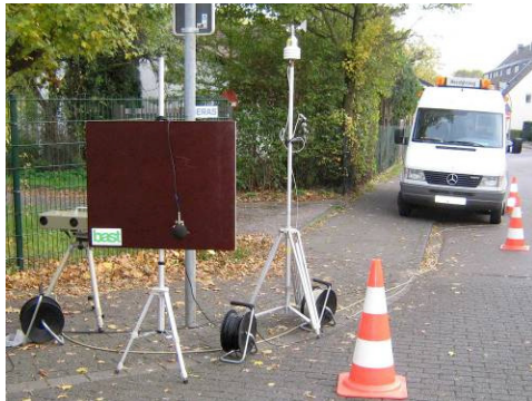
Figure 1: Backing Board (BB) at a measurement site in Cologne
