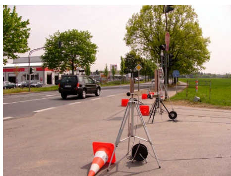
Figure 2: Measurement sites for SPB and CPB with Free Field (FF) and Backing Board (BB) at "Belgische Allee" in Cologne
