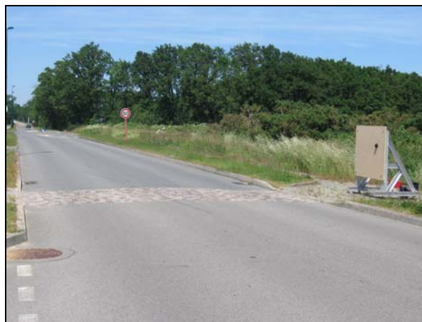
Figure 5 : Validation of the "Backing Board" technique a real discontinuity (pedestrian crossing)
