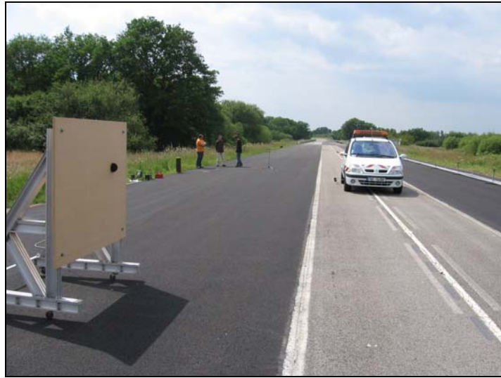
Figure 1 : Test vehicle passing-by the "Backing Board"
