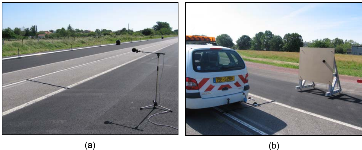
Figure 4 : Validation of the "Backing Board" technique on the LCPC Reference test track (a) the cable across the track; (b) the test vehicle passing on the cable
