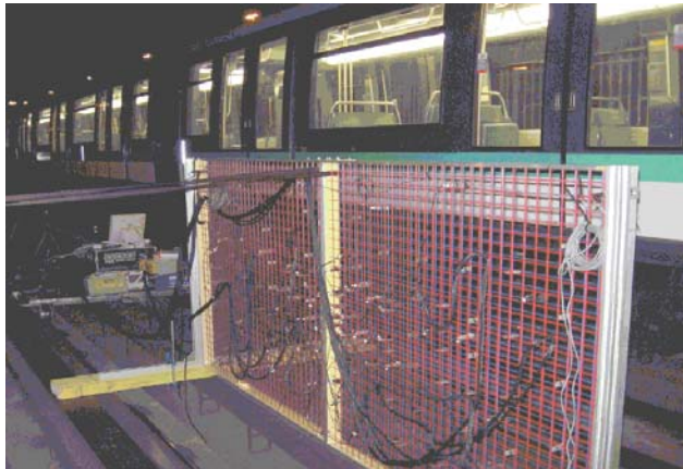
Antenna of 64 microphones to achieve the source ranking of a metro during its pass-by in normal operating conditions
