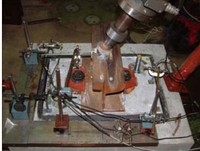
Fatigue testing of the innovative rail fastening system for trams
