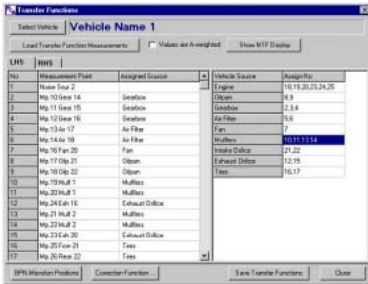
Picture 3: Assigning microphone measurements during operation to different sources
