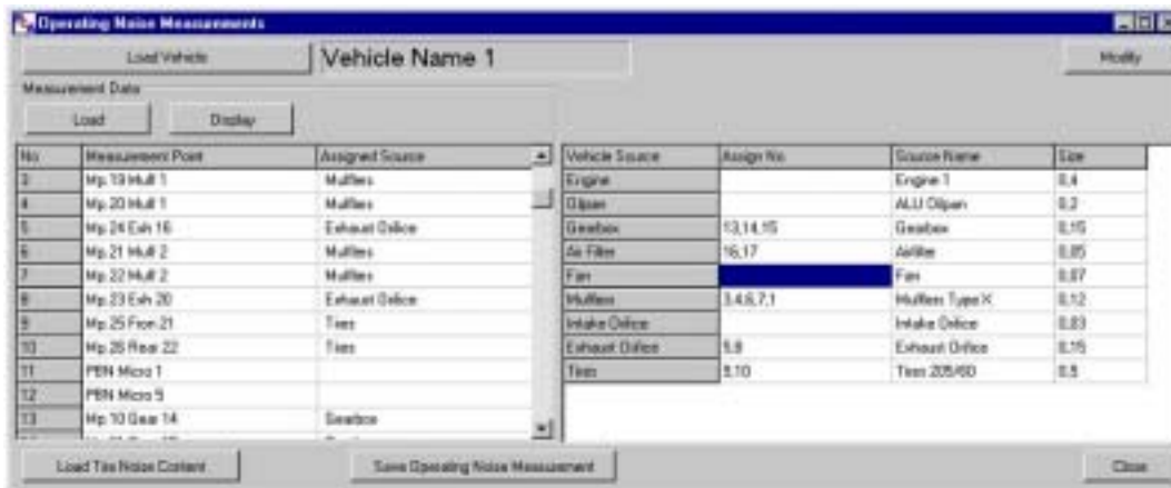
Picture 3: Assigning microphone measurements during operation to different sources
